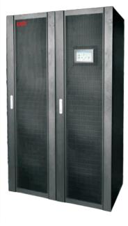
EA660 is the third generation of three phase high frequency on-line double-conversion modular UPS. Its single unit is extendable to 500 KVA / 450 KW, system capacity can be expanded to 2 MVA constructed by each module 50 KVA. All internal modules (Power module, bapass module and control module) are modularly designed and hot-swappable.
